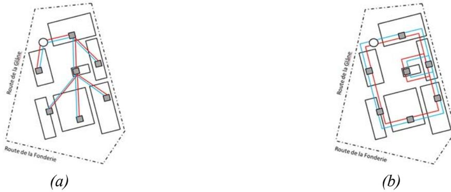
Fig. 1. BF potential network structures: a) Branched structure, b) Meshed structure
