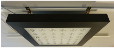
Figure 1. Prototype smart luminaire: an array of white LEDs mounted on actuators, behind an array of lenses. The actuators allow to direct the lights through the lenses for directional control.
